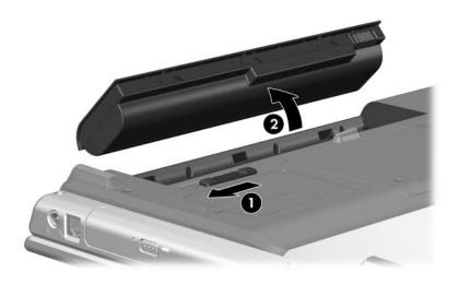
Removing the Battery Pack
